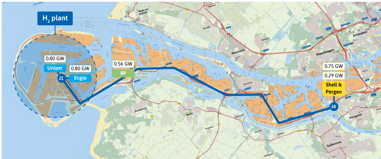
Figure 6.10: Reference scope case overview of the blue hydrogen production and transport infrastructure for the Rotterdam port, including both RFG and NG heating demand from end users. 'J#' are identifiers for junction points where the transmission pipeline splits into smaller lines going directly towards the plants.
